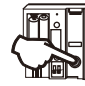
While pressing the test button Slide the on/off switch to 'on' position and hold the button 5 seconds. The LED will flash 5 times when a new code is generated
