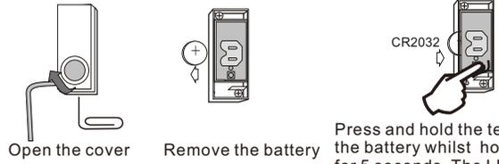
Press and hold the test button, insert the battery whilst holding the button for 5 seconds. The LED will flash 5 times when a new code is generated
